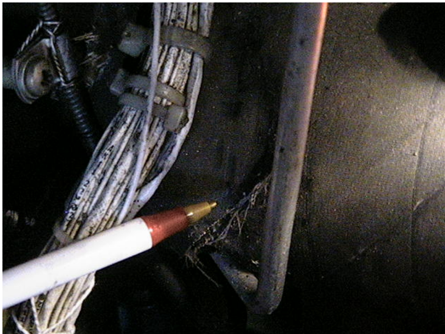
Figure 55. Damaged Air Inlet Pipe Due to Inadequate Clearance of the Wire Bundle in the Cessna 402C Forward Bulkhead Region
