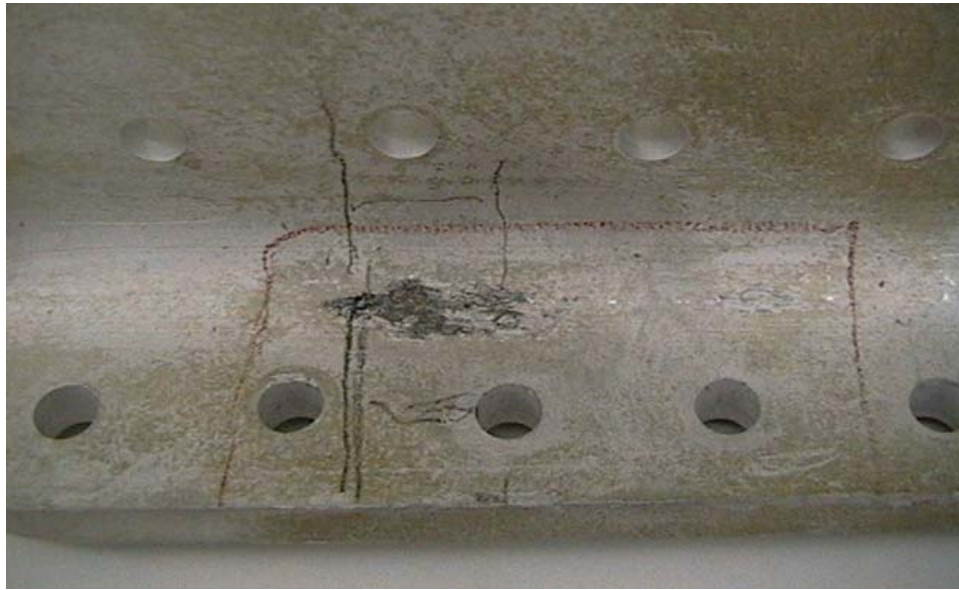
Figure 8. Moderate-Severe Corrosion on the Cessna 402A Left Wing Lower Front Fitting
