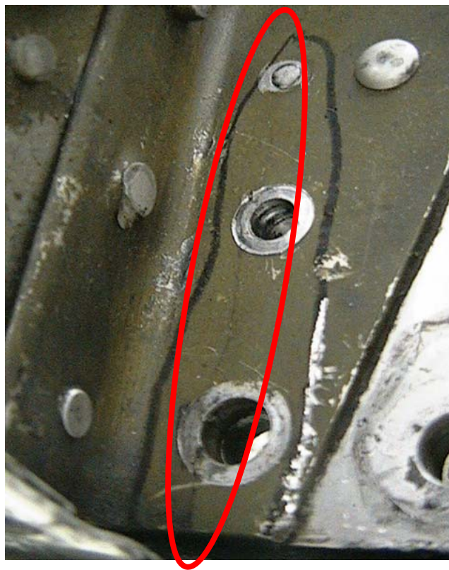
Figure 23. Crack in the Cessna 402C Angle Common to the Right Stub Wing Rib and Carry-Through Structure
