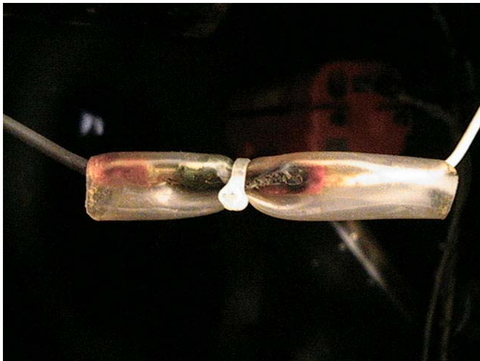
Figure 59. Heat-Damaged Wire in the Cessna 402C Tail Section
