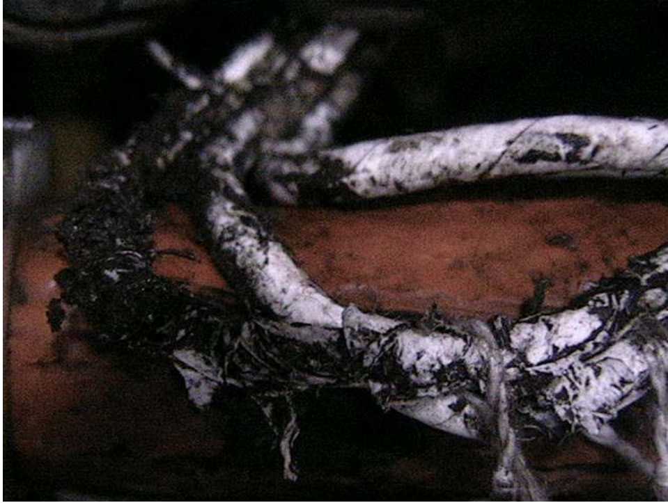
Figure 48. Worn and Dirty Wires in the Cessna 402C Right Engine Compartment
