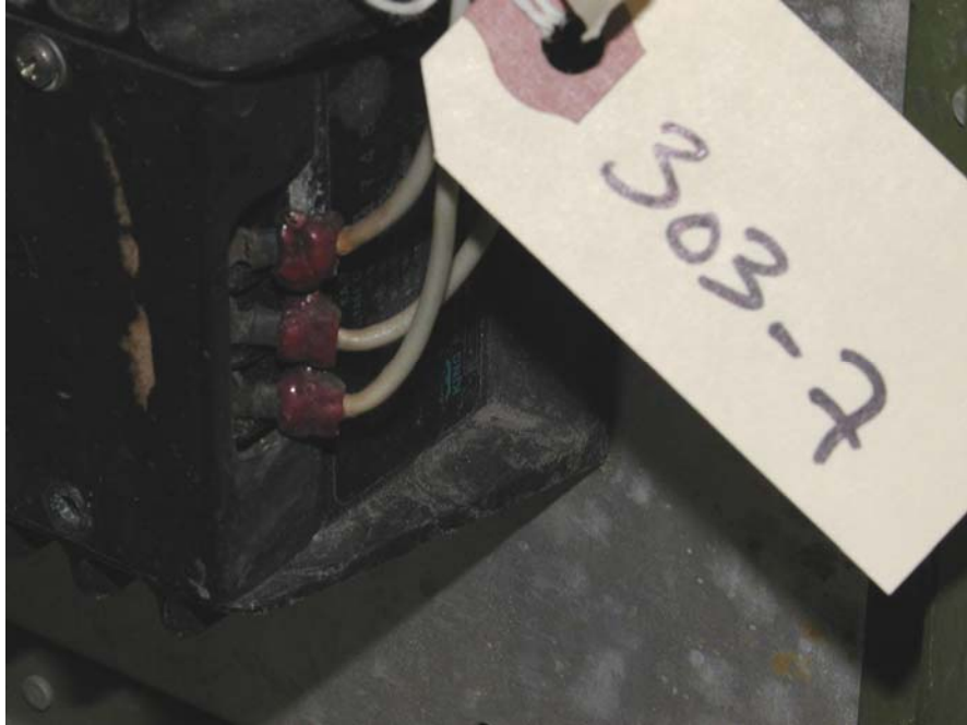
Figure 14. Heat-Damaged Terminals in the Cessna 402A Nose Compartment
