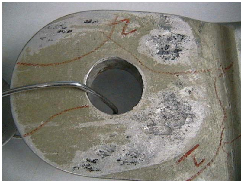
Figure 36. Area of Corrosion on the Cessna 402C Right Wing Forward Upper Attach Fitting
