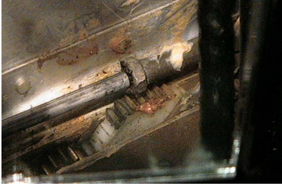
Figure 4. Broken Teeth on the Cessna 402A Left Fuel Selector Valve
