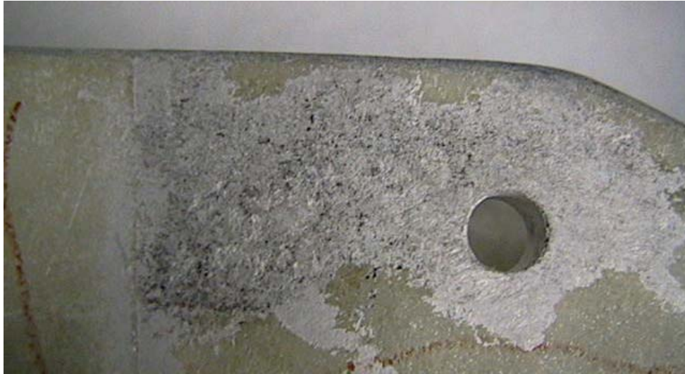
Figure 35. Area of Corrosion on the Cessna 402C Right Stub Wing Forward Upper Attach Fitting
