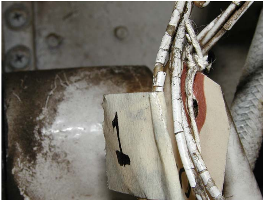
Figure 15. Cracked Wires in the Cessna 402A Landing Gear
