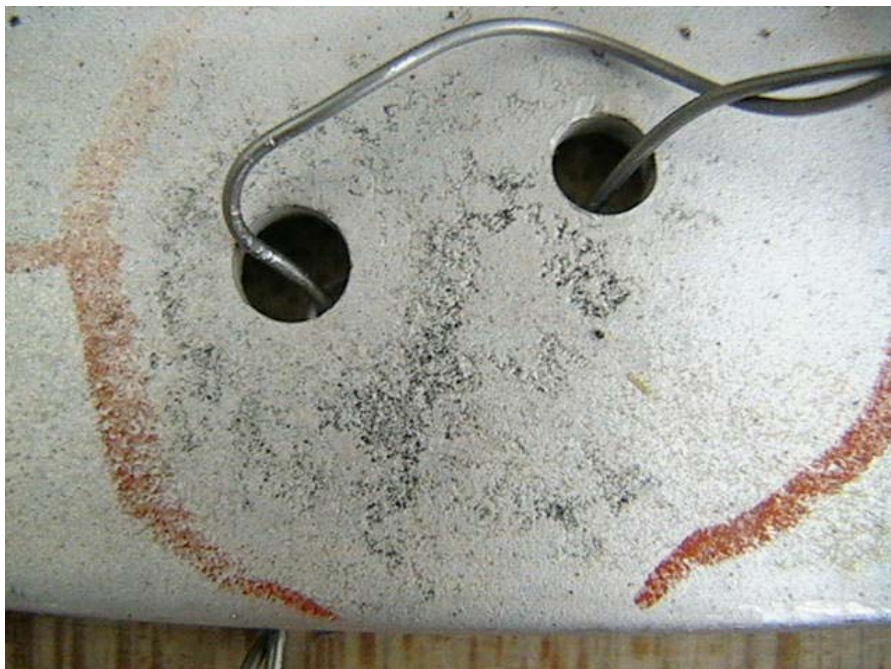
Figure 47. Corrosion on the Cessna 402C Horizontal Stabilizer Rear Spar Lower Cap
