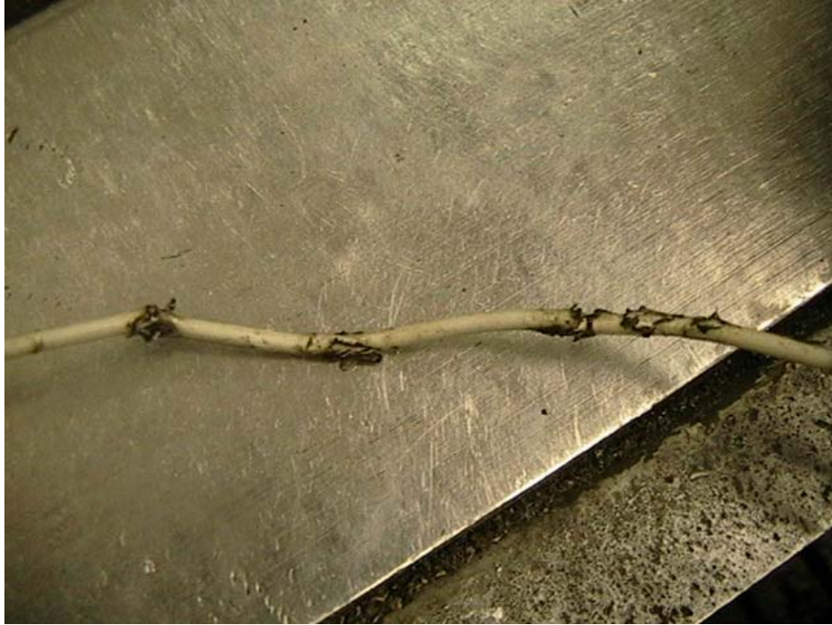
Figure 60. Cracked Insulation in the Cessna 402C Cockpit Floor
