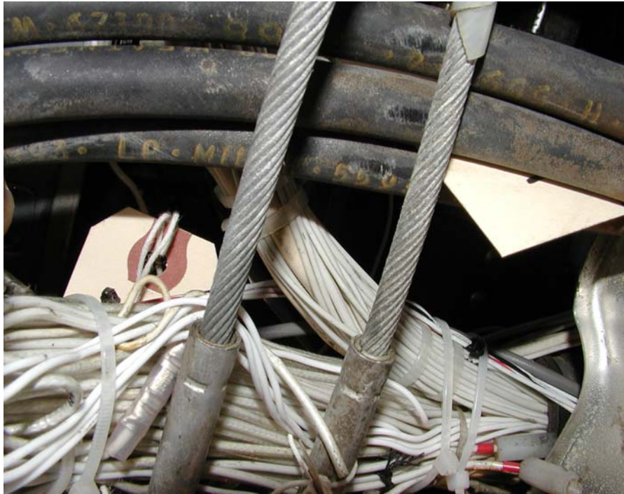
Figure 16. Wire Bundles Riding on the Cessna 402A Control Cables
