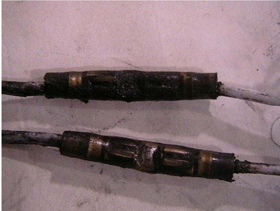
Figure 52. Grease Contamination at the Splices in the Cessna 402C Left Engine Compartment
