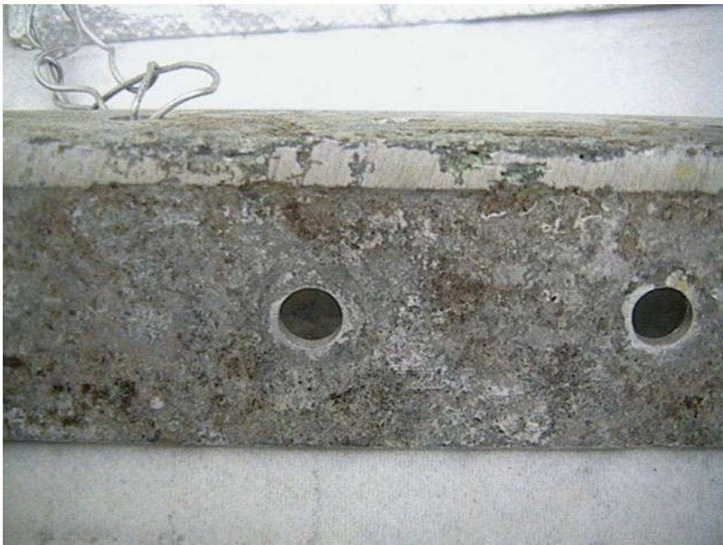
Figure 38. Area of Corrosion on the Cessna 402C Left Wing Rear Spar Lower Cap
