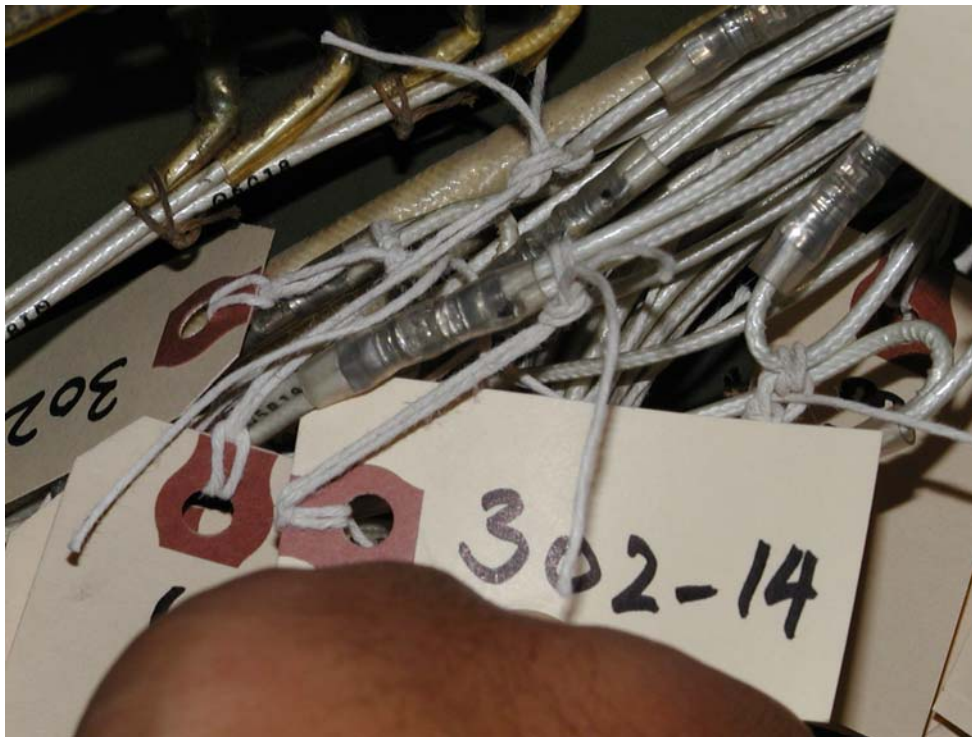
Figure 13. Repaired Wires in the Cessna 402A Side Console
