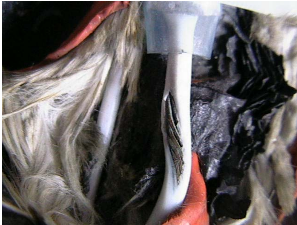
Figure 49. Exposed Inner Conductor in the Cessna 402C Right Engine Compartment
