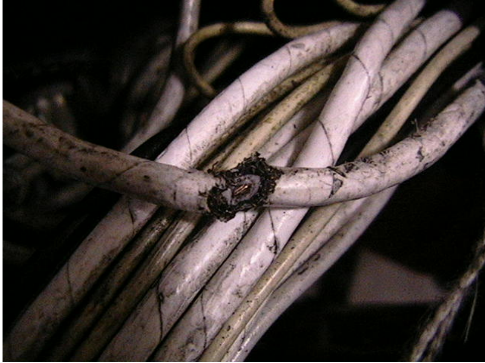
Figure 50. Damaged Shield Due to Cut Insulation in the Cessna 402C Right Engine Compartment
