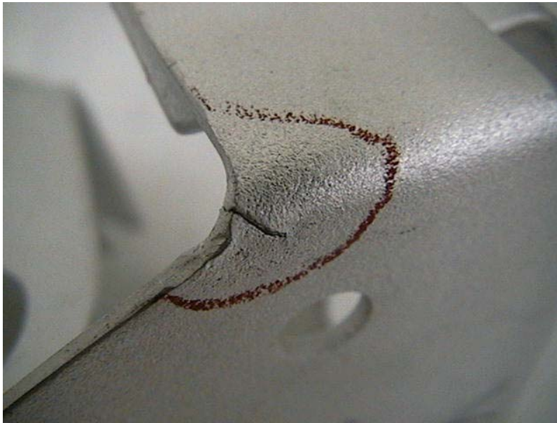
Figure 46. Crack on the Cessna 402C Left Inboard Elevator Attach Bracket
