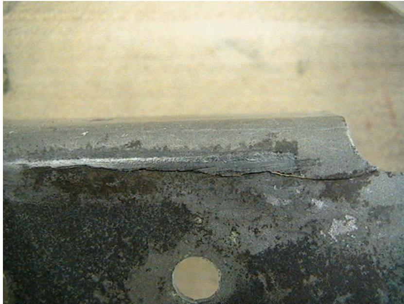
Figure 40. Crack on the Cessna 402C Left Wing Outboard Engine Beam
