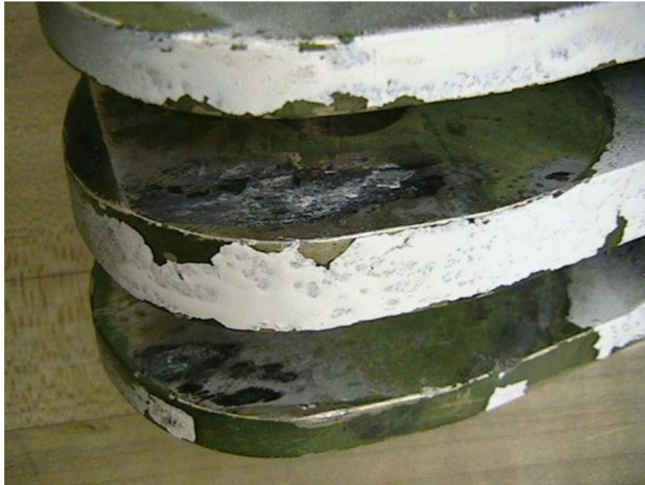
Figure 20. Corrosion Observed on the Cessna 402C Stub Wing Spar Attachment Fittings
