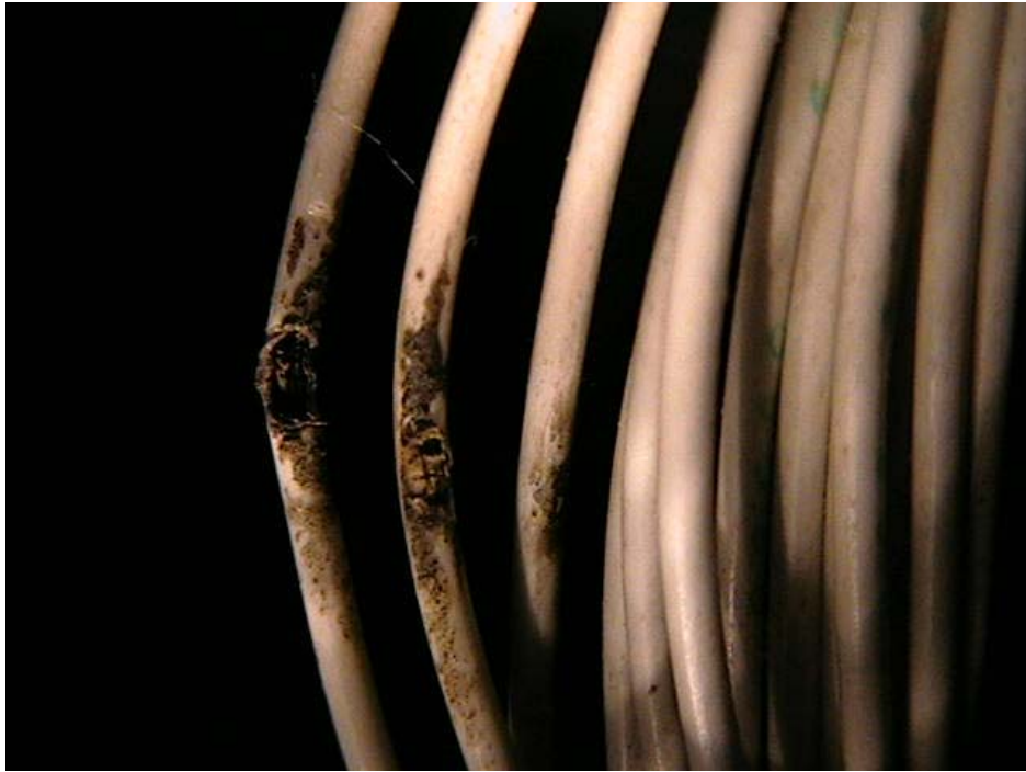
Figure 54. Heat-Damaged Inner Conductor in the Cessna 402C Right Console
