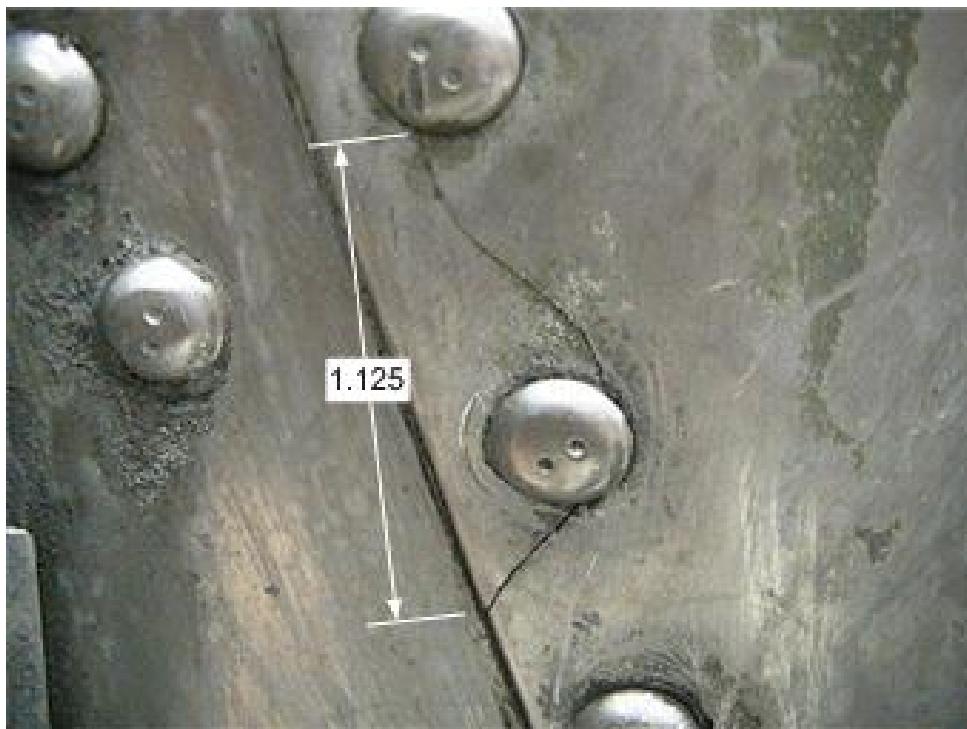
Figure 28. Cracked Cessna 402C Angle Bracket of the Right Wing Outboard Engine Beam
