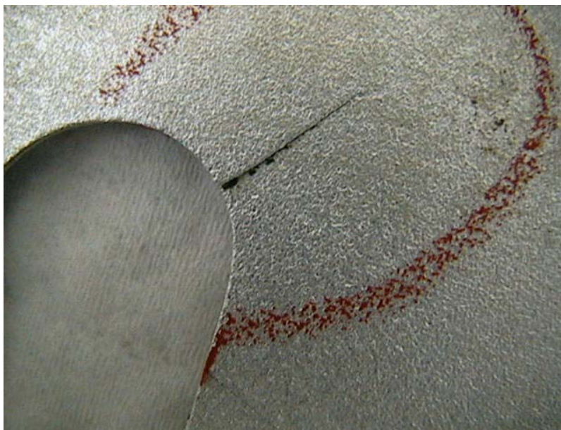
Figure 43. Crack in the Cessna 402C Carry-Through Aft Web
