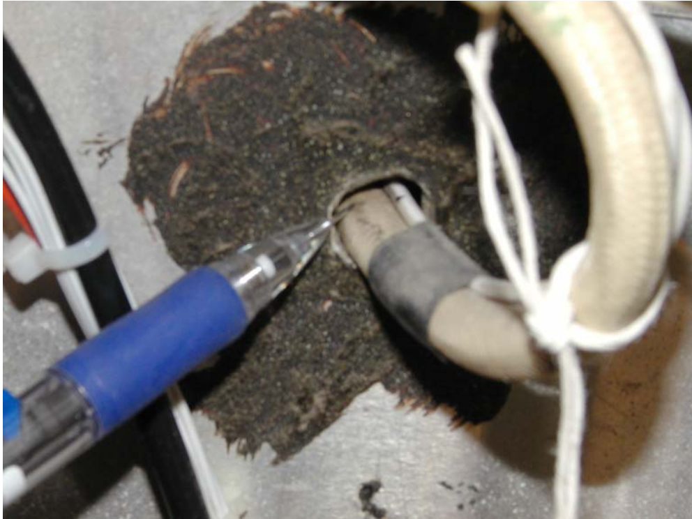
Figure 18. Missing Grommet Near Cessna 402A Upper Forward Bulkhead
