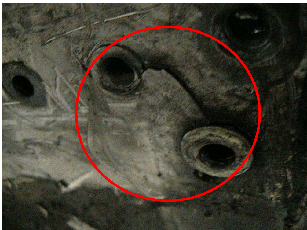
Figure 6. Crack on the Cessna 402A Right Wing Lower Skin
