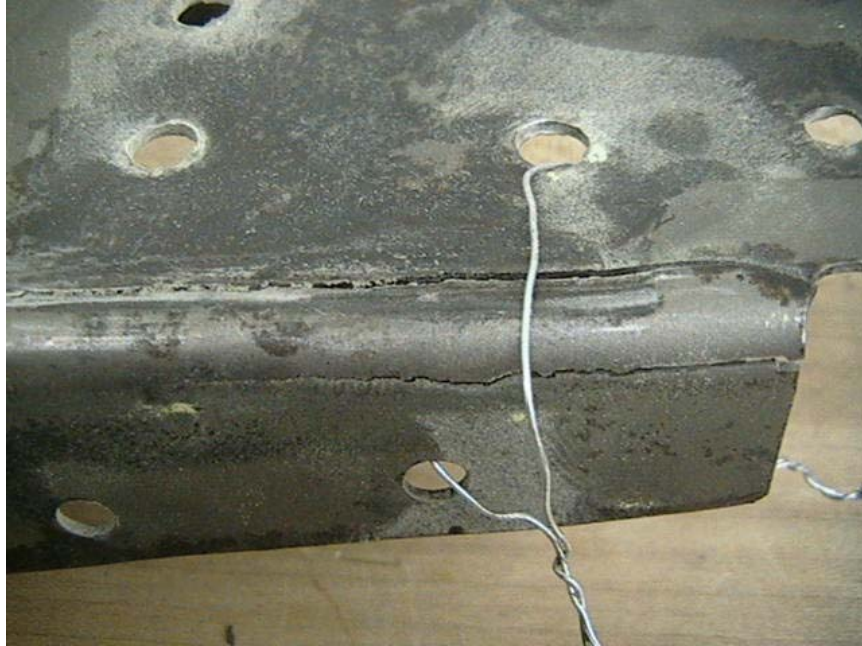
Figure 42. Crack in the Cessna 402C Right Wing Outboard Engine Beam
