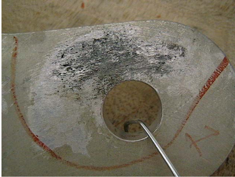
Figure 37. Area of Corrosion on the Cessna 402C Left Wing Lower Attach Fitting
