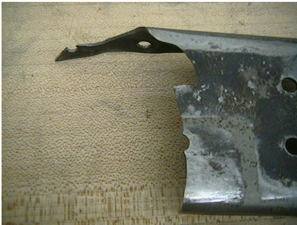
Figure 41. Crack Across Cessna 402C Right Wing Inboard Engine Beam
