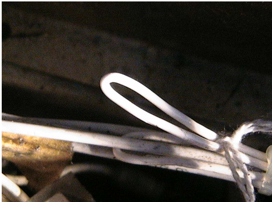
Figure 57. Improper Bend Radii Observed in the Cessna 402C Baggage Compartment
