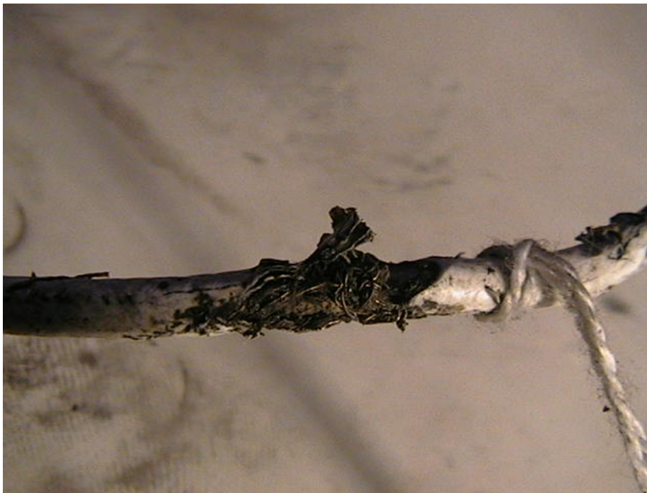
Figure 51. Damaged Outer Shield in the Cessna 402C Left Engine Compartment
