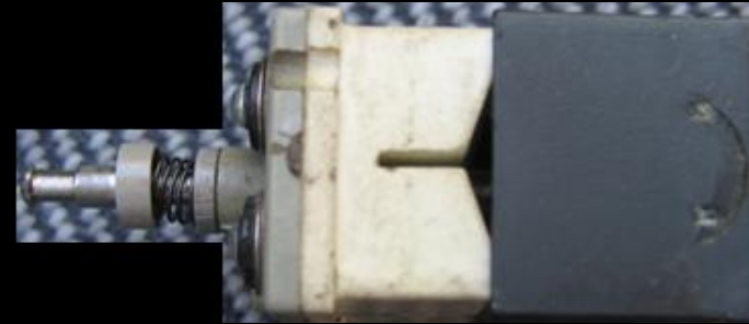
Gear indicator cube in extended position.
